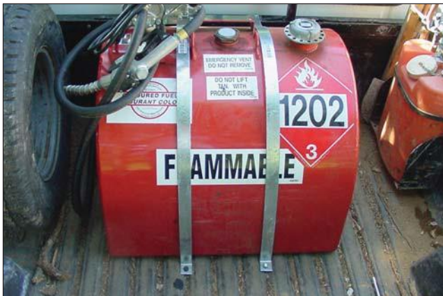
Fuel tank with appropriate markings and tiedowns.
