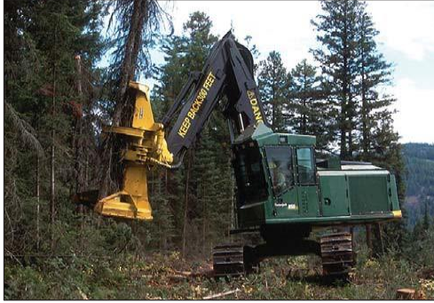
Feller buncher used in full tree harvest operation.
