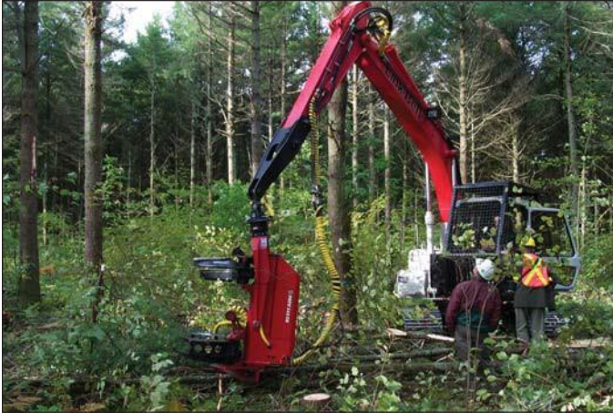
Processor used for commercial thinning .
